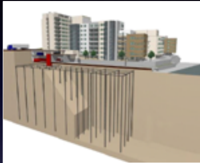
Ground storage for heating and cooling
